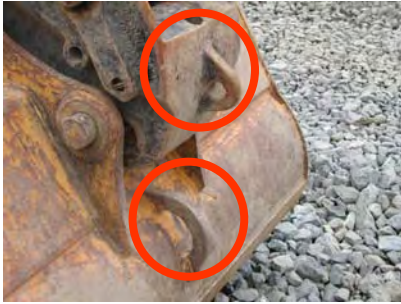
Lifting eyes mounted to the end of the stick and bucket.
