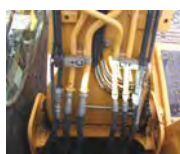
Check the hydraulic system, pumps, hoses, lines and cylinders, for leaks.
