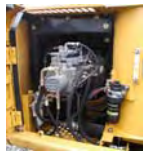
Check the hydraulic system, pumps, hoses, lines and cylinders, for leaks.
