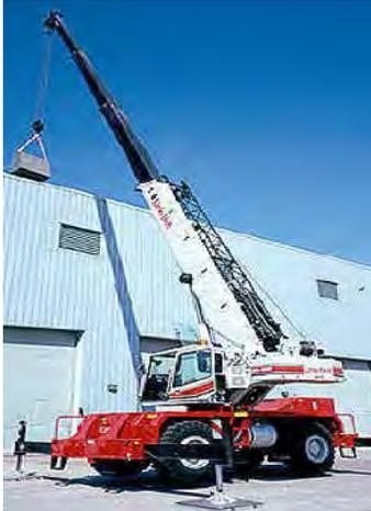
**BEFORE ATTEMPTING A LIFT, GATHER ALL NECESSARY INFORMATION ABOUT THE LOAD AND REFER TO THE LOAD CHART TO DETERMINE LIFT CAPACITY.**
