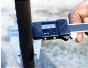
**MEASURE WIRE ROPE TO CHECK FOR WEAR**
