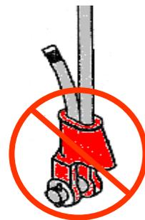
**LIVE WIRE MUST BE INSTALLED IN LINE WITH THE LOAD PIN**
