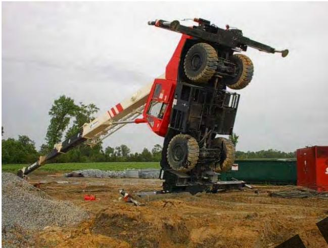
A major cause of crane accidents is the crane tipping over. The principles governing crane stability need to be clearly understood by the operator. Causes of tipover accidents are:
